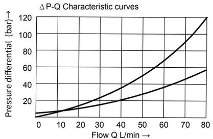
ΔP-Q- characteristic curve, flowing via one-way valve B to A.
